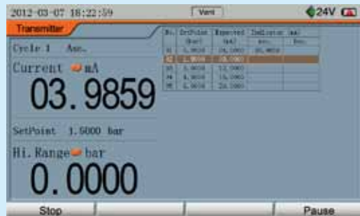
Pressure gauge / transmitter / switch calibration
